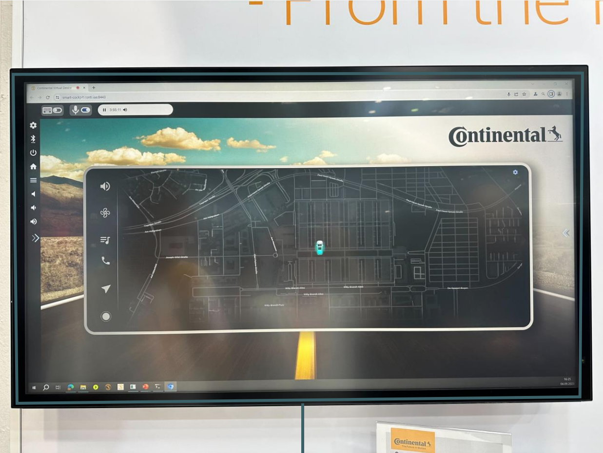
*Same* Android OS image running on Graviton, bi-directional UI streamed in browser through WebRTC
