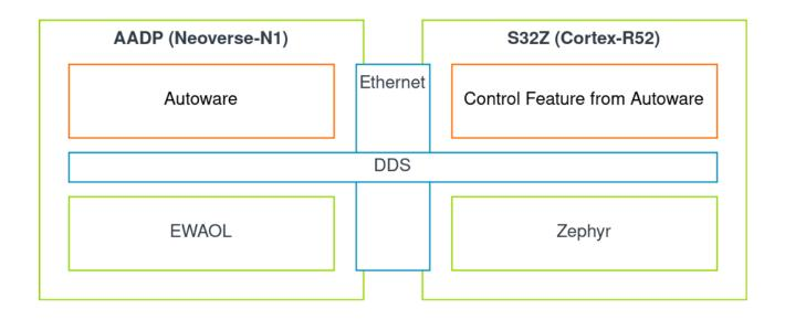
The software stack is deployed on the AADP (main compute) and the S32Z (critical compute)
