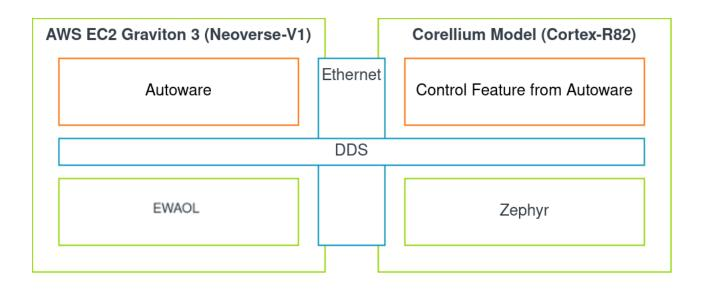
→ The software stack is deployed in the cloud using EC2 Graviton (main compute) and Corellium virtual hardware (critical compute)
